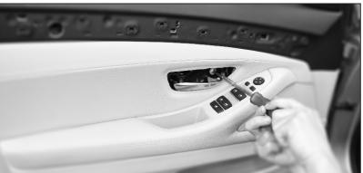
Note that the door panel is fixed by numerous plastic clips, carefully pry
